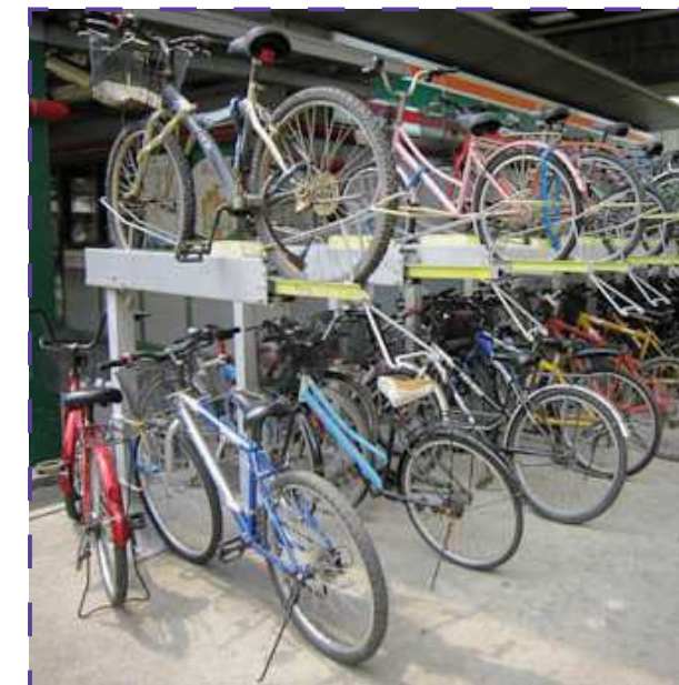
Sample covered double deck bicycle rack - for use in basement
